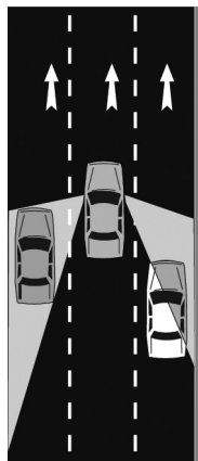
The accompanying diagram shows the "blind spots" around your vehicle, in which you cannot see with your vehicle's mirrors.
